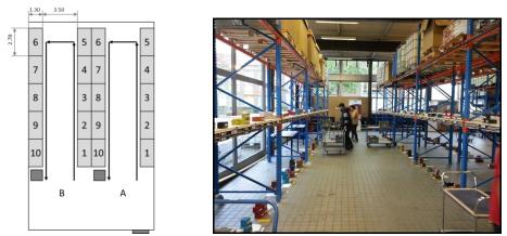
Figure 1: Experimental warehouse layout (measures are in meters).
